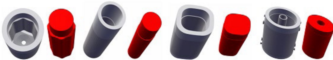
Figure 3: Ingot and molds generated by online Ingot Mold Design Assistant.
